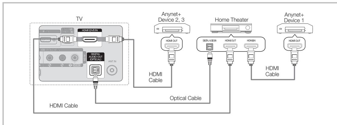
1. Connect the **HDMI (DVI) IN** jack on the TV and the **HDMI OUT** jack of the corresponding Anynet+ device using an HDMI cable.
